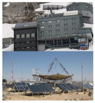
From the German Zugspitze to Israel's Negev desert, researchers at Fraunhofer ISE are investigating the aging of solar collectors and components under extreme climate conditions. ©Fraunhofer ISE
