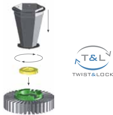
Solutions for LED module assembly
